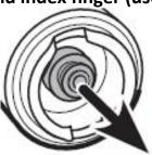
STEP FOUR: Insert new bulb in chamber in direction of arrow as shown below
